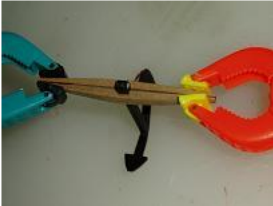
Anchor and pegs. The metal body is painted before the two parts of the stock are clamped and glued in place. There is a small gap between the two halves of the stock near the centre
